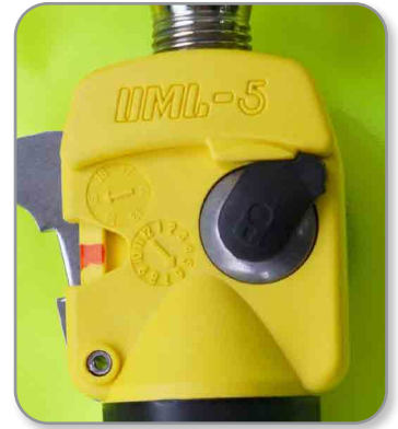
Plastic torx head cover placed over torx bolt
