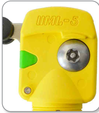
Uses a TX30 Torx Bolt A Torx adapter will be required to tighten the unit to 3nm
